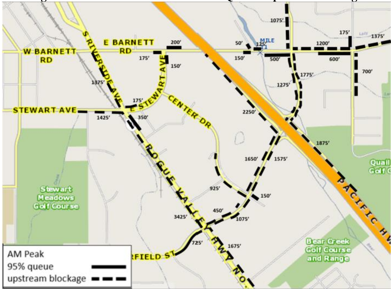
Figure 4 - Future Year 2045 AM Peak Queues/Upstream Blockage
